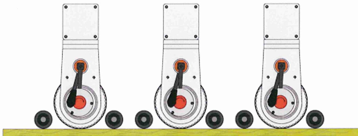
Top working, equipped with 3 texturing brush units.
